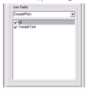
The drop down list allows you to select the layer from which fields should be copied across to the output transect shapefile. The checked list underneath allows you to interactively choose which fields should be copied across or not.
