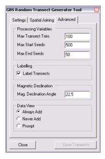
The GBS Transect Tool form is used to set any parameters and processing settings used during the generation of the random transects. The default values seen when the form opens are sourced from the GBS XML Configuration file (gbsConfig.xml) stored in the tools installation directory (or a network location if desired). These default values can be easily changed in a text editor and steps to do so will be described in a later section.
